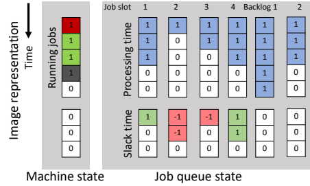
Fig. 2: State representation: this state looks T = 5 time steps ahead of current time and slack time array length is Z = 3 ; there are n = 4 job slots and m = 10 backlog slots. The machine state (schedule of next T time steps) tells that the next 4 time steps have been scheduled. For the job in job slot 1, p = 3 , slack = 1 ; for the job in job slot 3, p = 2 , slack = -1 . There are 8 jobs waiting in backlog. Different colors in machine state represent different jobs.
